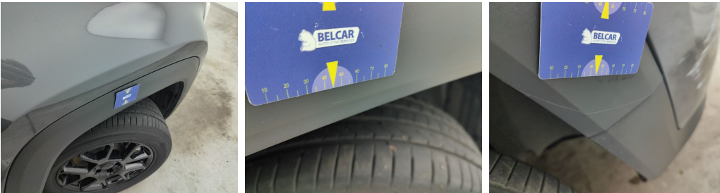
Wing Front right / Trim / Replace-scratch
