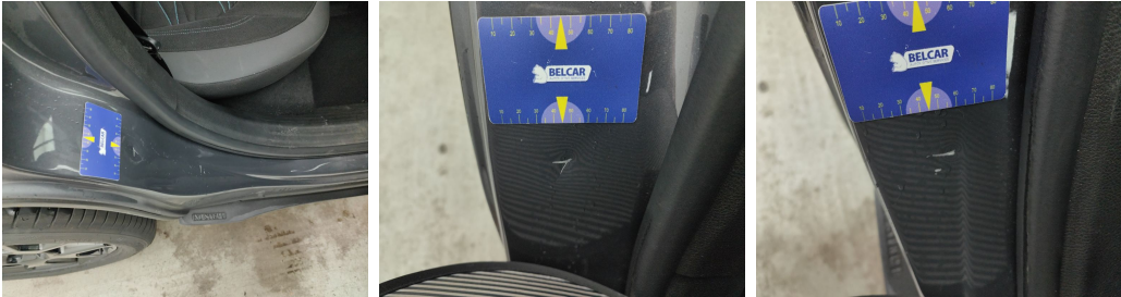
Rocker Panel Right // Smart Repair Medium-scratch + dent
