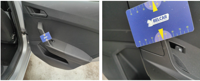
Rear Right Door Interior Coating / Door Handle / Replace-scratch
