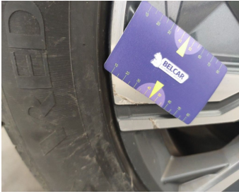
Wheel Two Tone Rear Right // Repair-scratch
