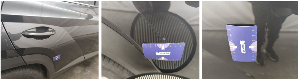
Door Rear Right // Repair & Painting-scratch + dent
