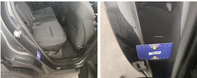
Rocker Panel Right // Smart Repair Medium-scratch + dent
