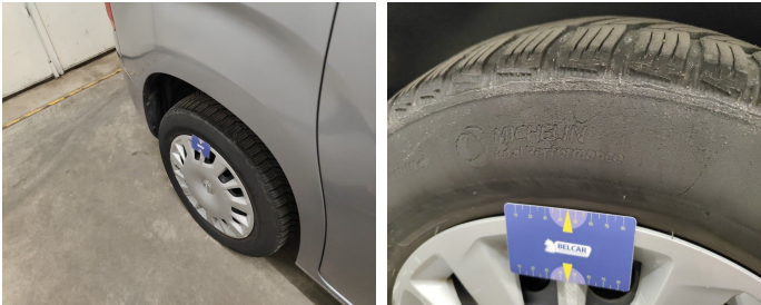
Tyre Rear Right // Replace-worn
