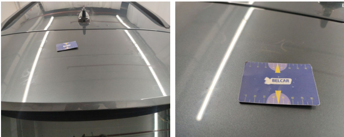
Rear Bonnet // Smart Repair Large-Chemical reaction
