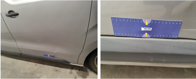
Door Front Right / Trim / Replace-scratch
