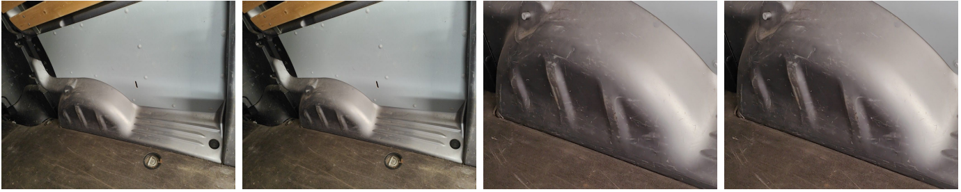
Trunk Compartment // Repair-scratch
