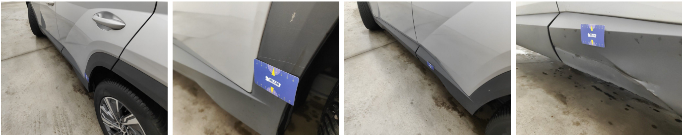
Door Rear Left / Trim / Replace-scratch + dent
