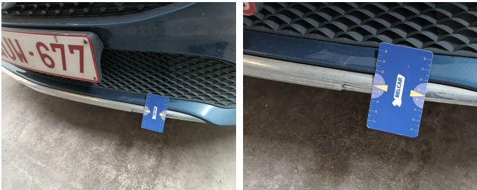
Bumper Front / Spoiler / Replace-cracked
