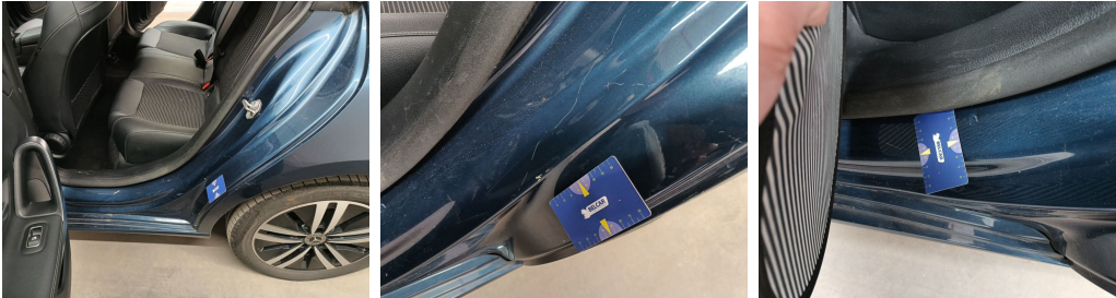
Rocker Panel Left // Smart Repair Medium-scratch + dent
