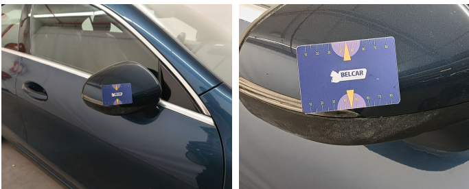
Side View Mirror Right / Direction Indicator / Replace-cracked
