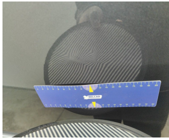
Wing Rear Left // Repair & Painting-dent
