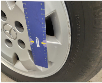
Wheel Alloy Front Left // Repair-scratch
