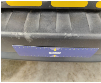
Bumper Rear / Lower Cover Not Painted / Replace-scratch
