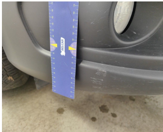
Bumper Front / Lower Cover Not Painted / Replace-scratch
