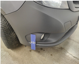
Bumper Front / Lower Cover Not Painted / Replace-scratch
