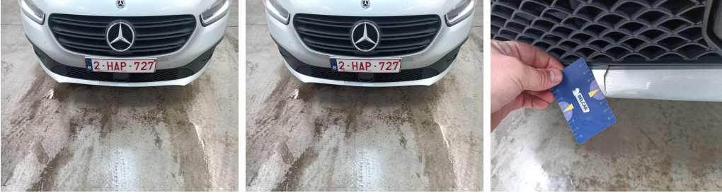
Bumper Front // Replace & Painting-cracked
