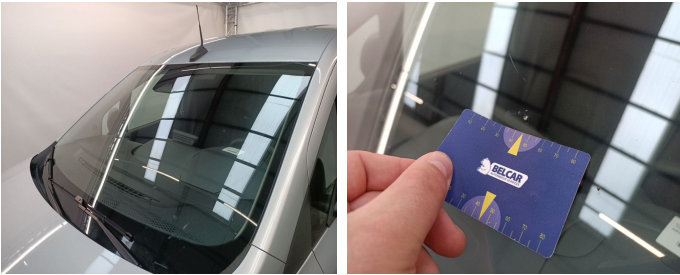
Windshield // Replace-glass damage
