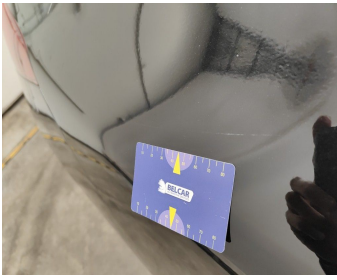
Wing Rear Right // Polish-scratch
