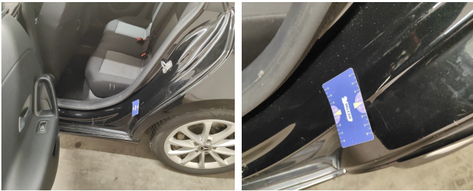
Rocker Panel Left // Painting-scratch
