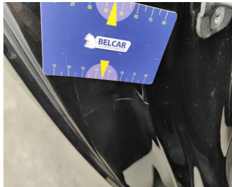
Rocker Panel Right // Painting-scratch
