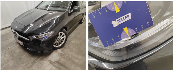
Headlight / Front left / Replace-scratch
