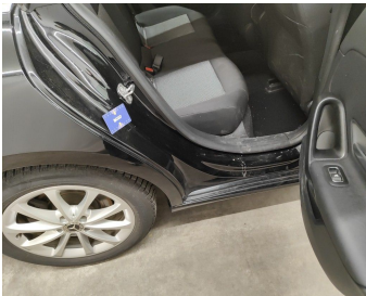
Rocker Panel Right // Painting-scratch
