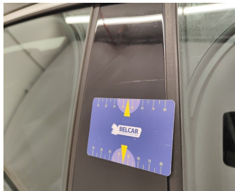
Door Front Right / Trim / Replace-scratch
