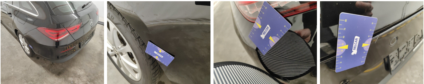
Bumper Rear // Painting-bad repair
