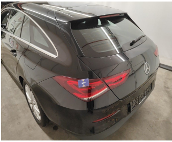
Light / Rear left / Replace-scratch
