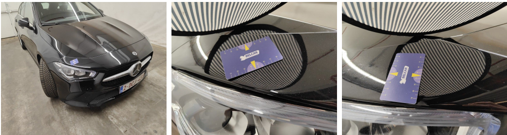
Bumper Front // Painting-bad repair
