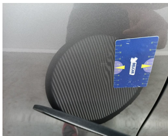
Door Front Right // Smart Repair Small-scratch + dent
