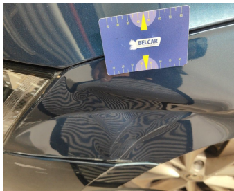
Wing Front Left // Repair & Painting-scratch + dent
