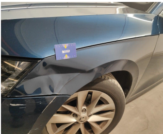
Wing Front Left // Repair & Painting-scratch + dent
