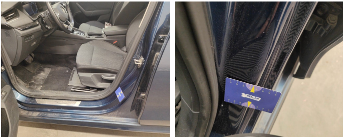
Rocker Panel Left // Smart Repair Medium-dent
