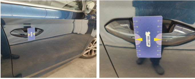
Door Front Right // Smart Repair Small-scratch
