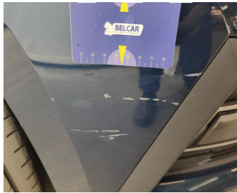
Bumper Front // Replace & Painting-scratch + dent
