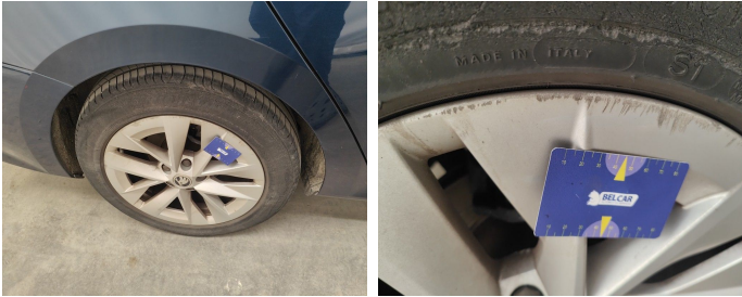
Wheel Alloy Rear Right // Repair-scratch
