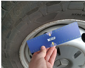
Wheel Steel Front Left // Replace-rust
