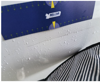
Door Rear Right // Repair & Painting-scratch + dent
