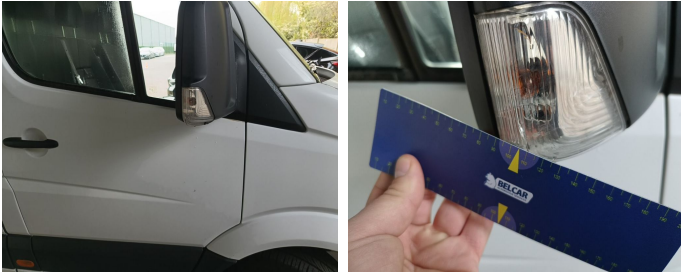
Side View Mirror Right / Direction Indicator / Replace-cracked
