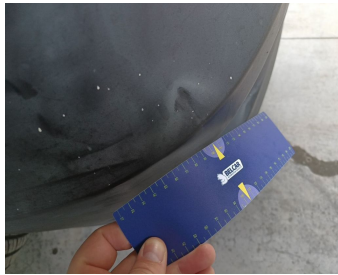
Wing Front right // Repair & Painting-scratch + dent
