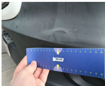
Bumper Front // Replace without painting-scratch + dent
