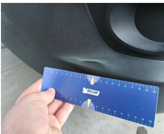
Bumper Front // Replace without painting-scratch + dent
