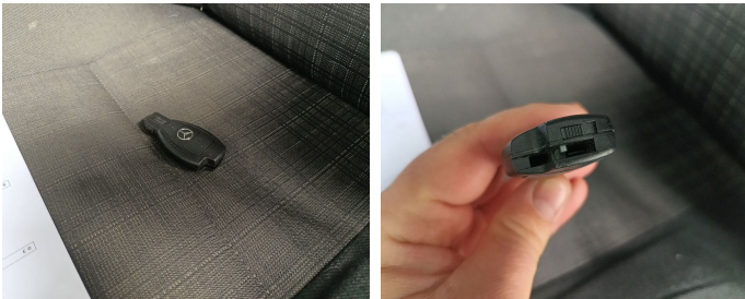
Emergency Key //-missing
