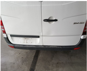
Rear Loading Door Right // Repair & Painting-cracked
