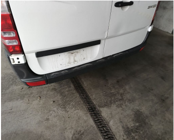
Bumper Rear // Replace without painting-scratch + dent
