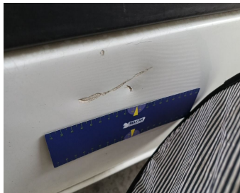
Door Front Right // Repair & Painting-scratch + dent
