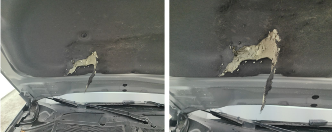
Front Bonnet / Insulation / Replace-tear
