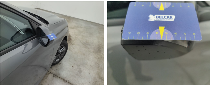
Damage within Renta-norm-scratch
