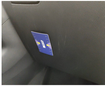
Dashboard / Cover Storage Tray / Replace-scratch
