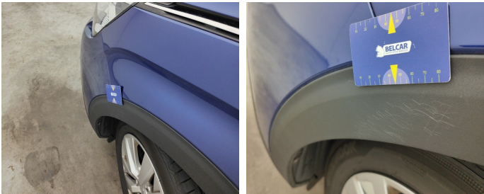
Wing Front Left / Trim / Replace-scratch
