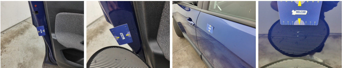
Door Rear Left // Repair & Painting-dent
