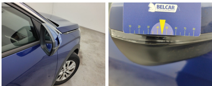
Side View Mirror Right / Direction Indicator / Replace-scratch
