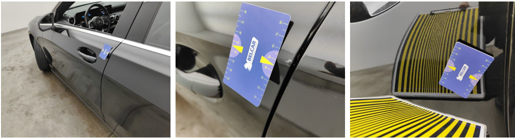
Door Front Left // Painting-bad repair
