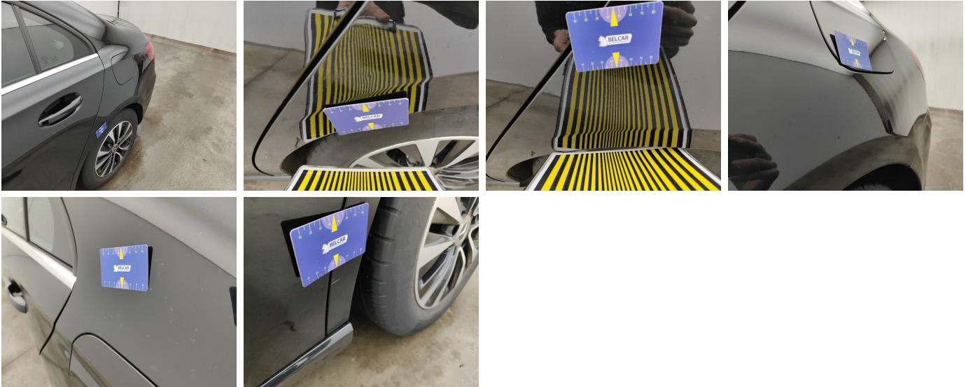
Wing Rear Left // Painting-bad repair
