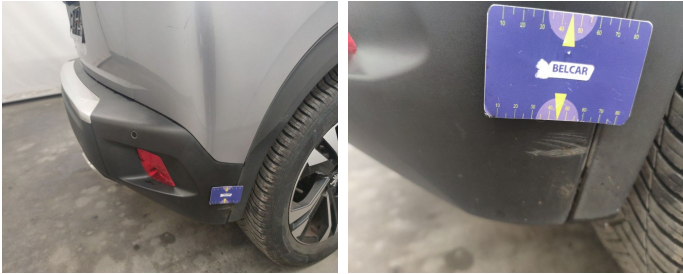
Bumper Rear / Lower Cover Not Painted / Replace-scratch
