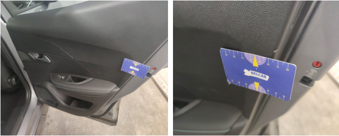
Rear Right Door Interior Coating // Replace Completely-scratch
