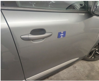
Door Front Right // Repair & Painting-scratch + dent
