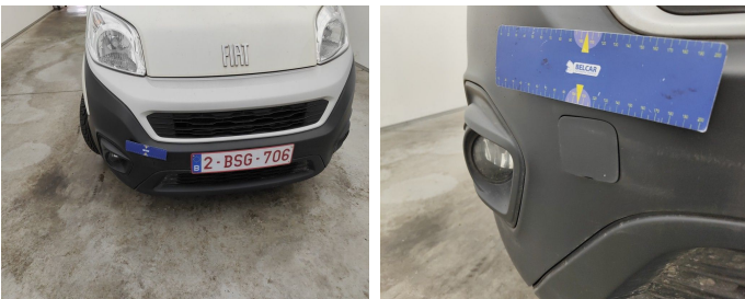
Front / Towing Cover / Replace-bad position
