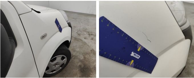
Wing Front right // Painting-scratch
