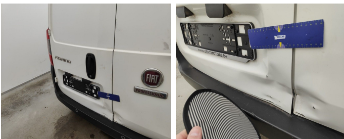
Rear Loading Door Left // Repair & Painting-scratch + dent
