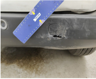
Bumper Rear / Lower Cover Not Painted / Replace-hole
