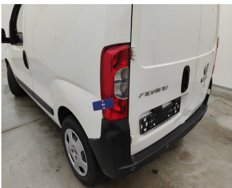
Light / Rear left / Replace-cracked
