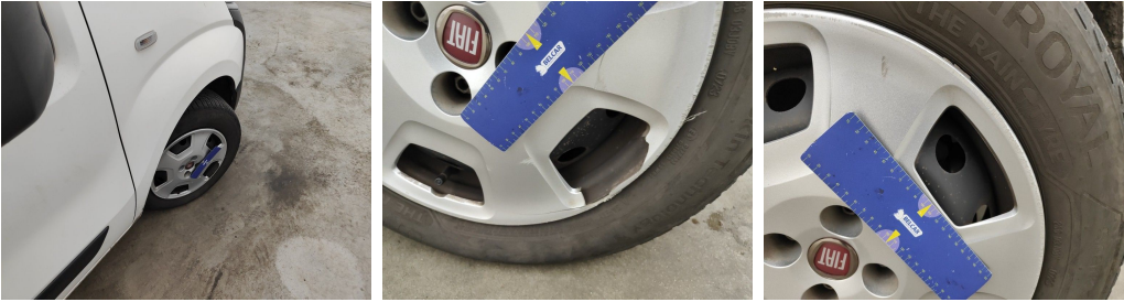
Wheel Front Right / Wheel Cover / Replace-cracked
