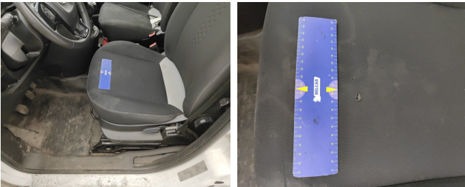
Seat Front Left / Bottom Coating / Replace-Incinerated
