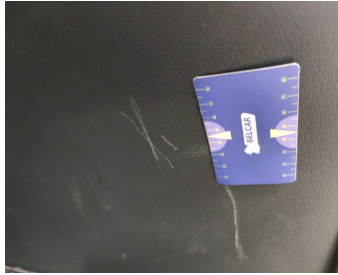
Wing Front Left // Smart Repair Medium-scratch
