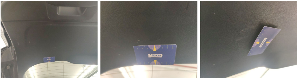
Trunk Lid Interior Coating / Complete Panel / Replace-scratch
