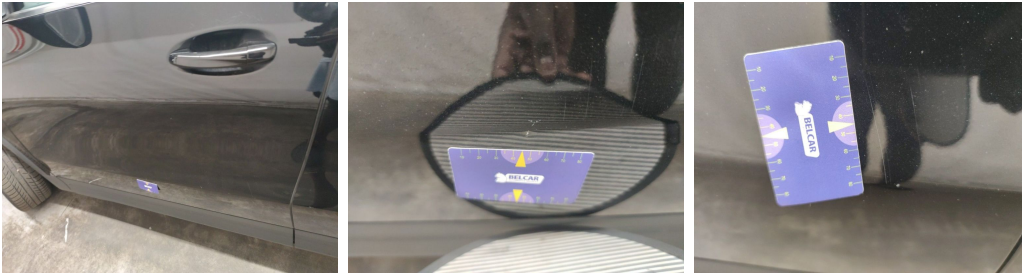
Rocker Panel Left // Smart Repair Medium-dent
