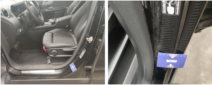
Rocker Panel Left // Smart Repair Medium-dent
