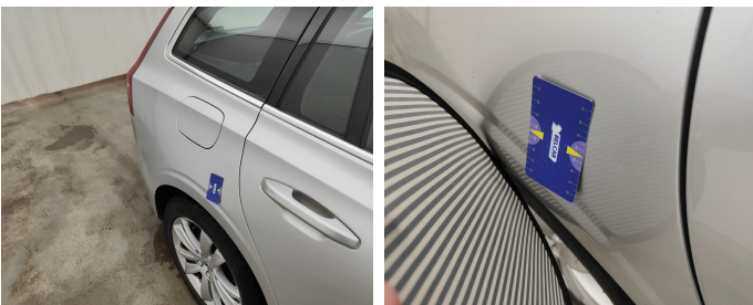
Wing Rear Right // Repair & Painting-scratch + dent
