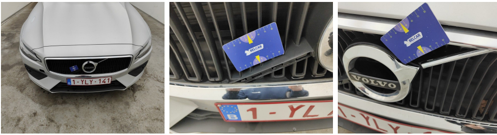
Front / Logo / Replace-cracked
