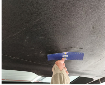
Trunk Lid Interior Coating / Complete Panel / Replace-scratch
