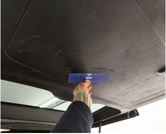
Trunk Lid Interior Coating / Complete Panel / Replace-scratch
