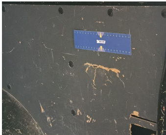
Trunk Compartment / Side Cover Right / Replace-cracked
