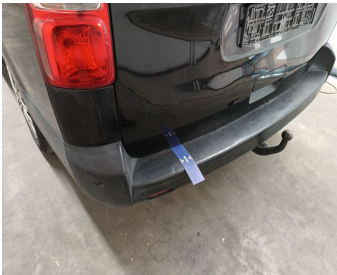
Bumper Rear // Replace without painting-scratch + dent
