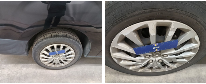
Wheel Rear Right / Wheel Cover / Replace-Chipped paint
