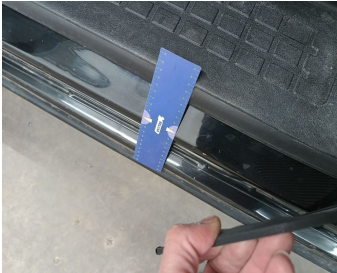
Rocker Panel Right // Smart Repair Medium-scratch + dent
