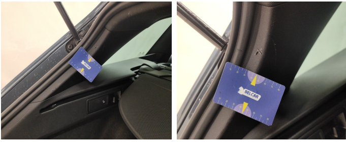
Trunk Compartment / Side Cover Left / Replace-scratch
