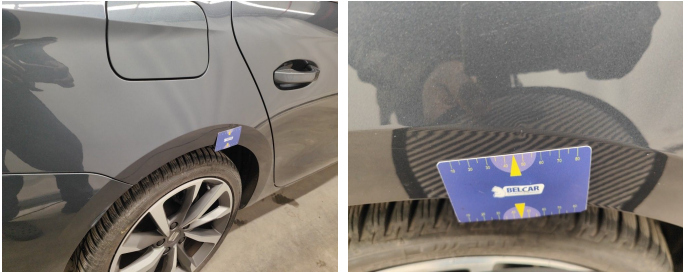
Wing Rear Right // Repair & Painting-scratch + dent
