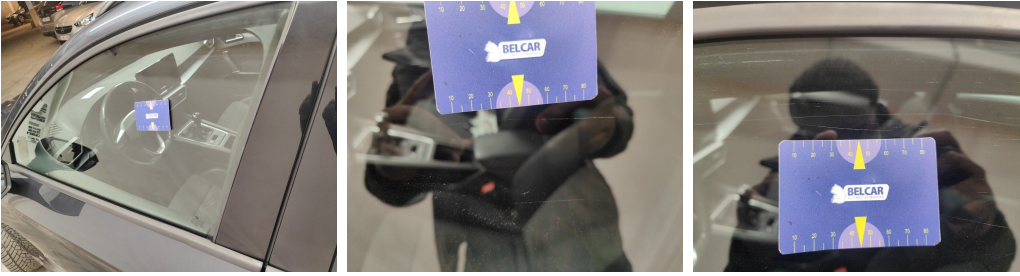
Door Front Left / Window / Replace-scratch
