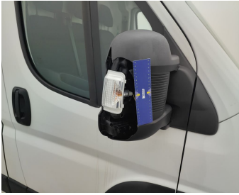
Side View Mirror Right // Replace Not Painted-cracked
