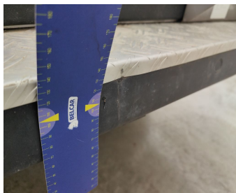
Bumper Rear / Trim Center / Replace-scratch + dent
