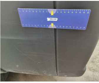
Bumper Rear // Replace without painting-scratch + dent
