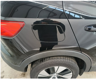
Wing Rear Right / Fuel Cover / Replace-scratch
