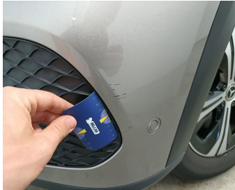
Bumper Front // Smart Repair Medium-scratch
