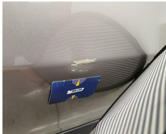
Door Front Right // Repair & Painting-scratch + dent
