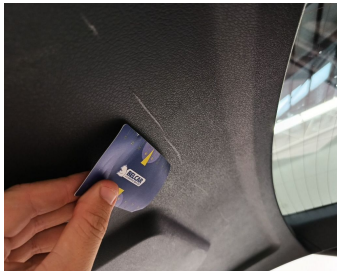
Trunk Lid Interior Coating / Complete Panel / Replace-scratch
