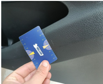
Front Right Door Interior Coating // Replace Completely-scratch
