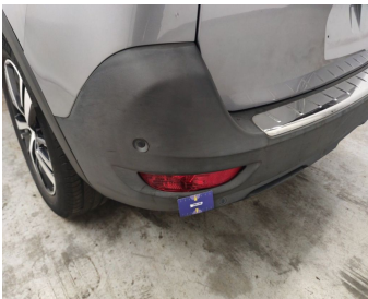
Foglight Rear // Replacement-cracked
