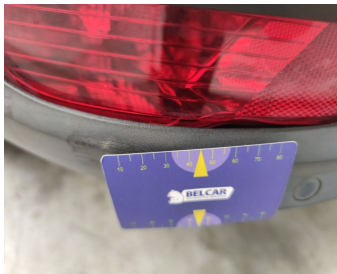
Foglight Rear // Replacement-cracked
