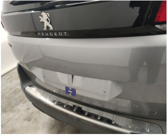
Rear Bonnet // Smart Repair Small-dent
