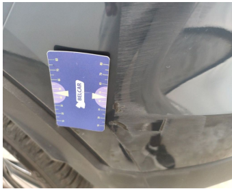
Bumper Rear / Lower Cover Not Painted / Replace-scratch
