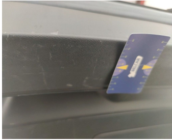
Trunk Lid Interior Coating / Complete Panel / Replace-scratch
