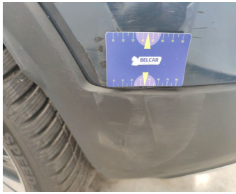
Bumper Rear / Lower Cover Not Painted / Replace-scratch
