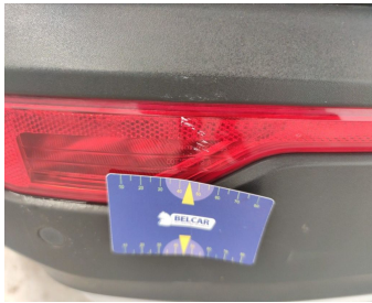
Back Side / Reflector L / Replace-scratch
