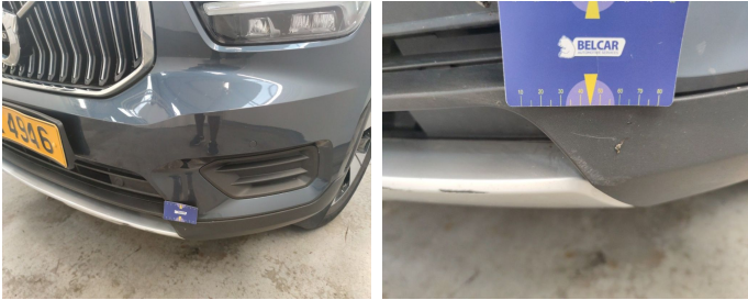
Bumper Front / Lower Cover Not Painted / Replace-scratch
