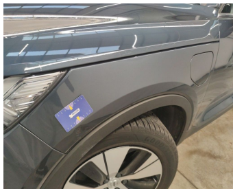
Wing Front Left // Repair & Painting-scratch + dent
