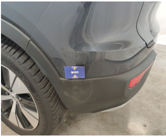
Bumper Rear / Lower Cover Not Painted / Replace-scratch
