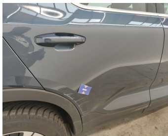
Door Rear Right // Repair & Painting-scratch + dent
