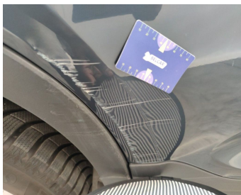
Door Rear Right // Repair & Painting-scratch + dent
