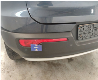
Back Side / Reflector L / Replace-scratch
