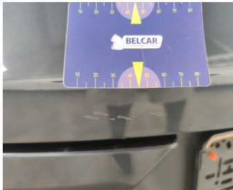
Trunk Lid Interior Coating / Complete Panel / Replace-scratch
