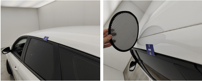
Roof // Smart Repair Medium-dent
