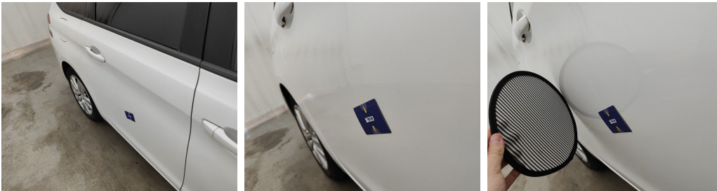
Door Rear Right // Painting-bad repair
