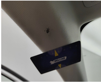
Interior / Headliner/ Replace-Incinerated
