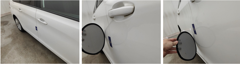
Door Front Right // Repair & Painting-dent
