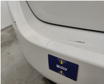
Bumper Rear // Replace & Painting-cracked
