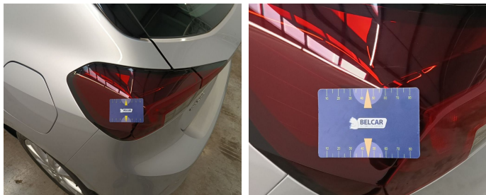
Light / Rear left / Replace-scratch
