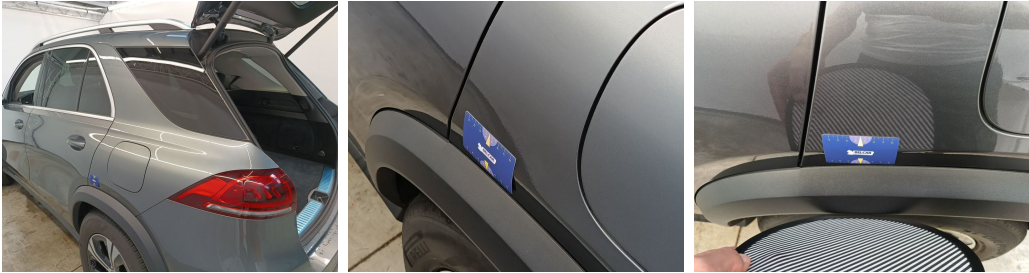
Wing Rear Left // Smart Repair Small-dent
