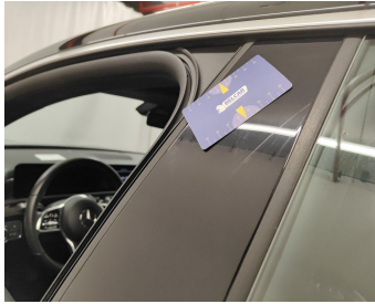
Door Front Left / Trim / Replace-scratch
