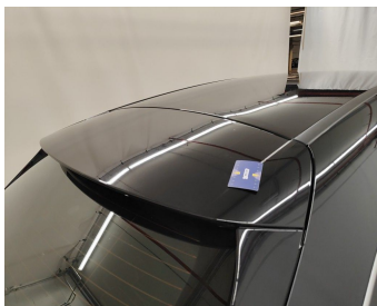
Rear Bonnet / Spoiler / Replace & Painting-scratch
