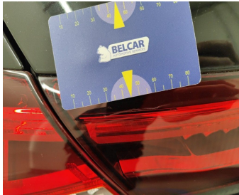
Light / Rear Left On Rear Bonnet / Replace-scratch
