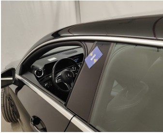
Door Front Left / Trim / Replace-scratch
