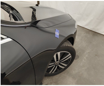
Wing Front right // Polish-scratch
