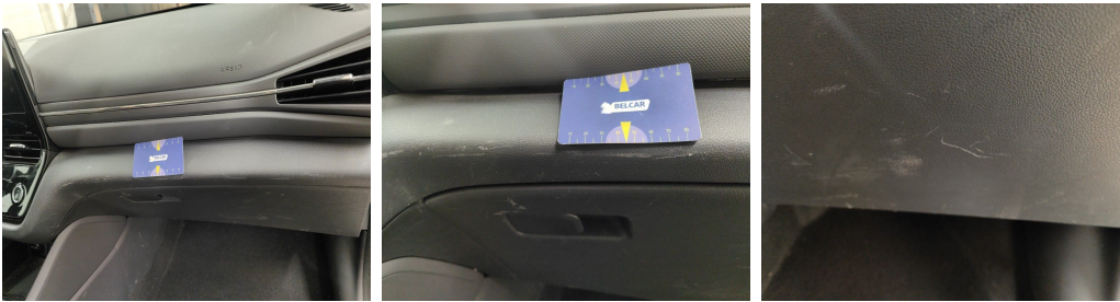
Dashboard // Replace Completely-scratch
