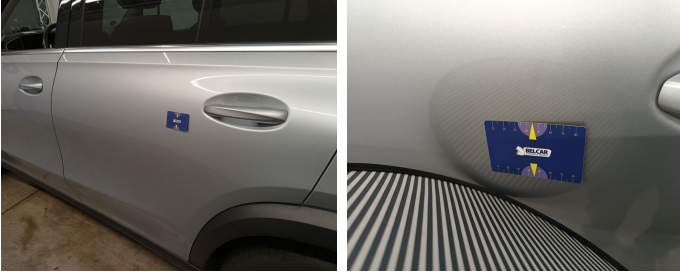
Damage within Renta-norm-dent
