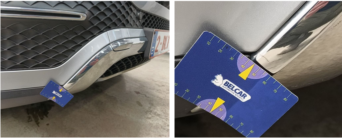
Bumper Front / Lower Cover Not Painted / Replace-cracked
