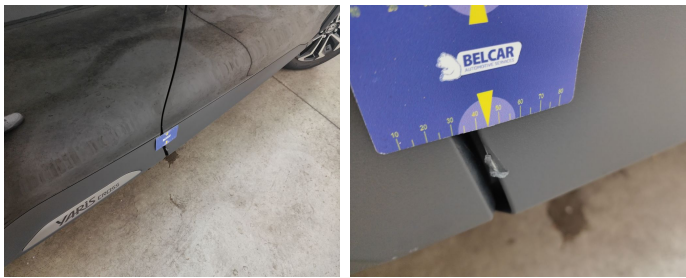
Door Front Right / Trim / Replace-scratch
