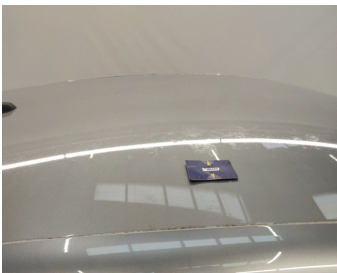
Roof // Polish-Chemical reaction
