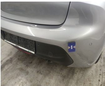
Bumper Rear // Painting-scratch
