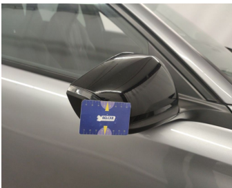
Side View Mirror Right // Painting-scratch
