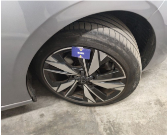
Tyre Front Right // Replace-tear
