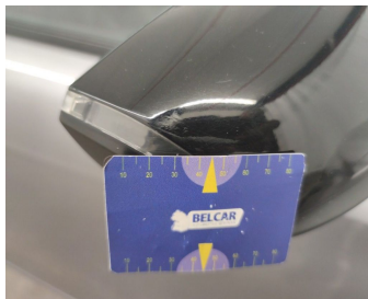
Side View Mirror Right // Painting-scratch
