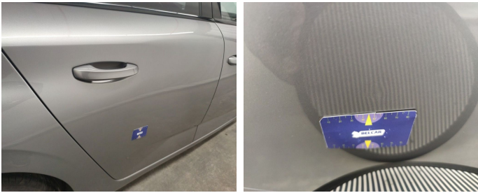
Door Rear Right // Smart Repair Small-dent
