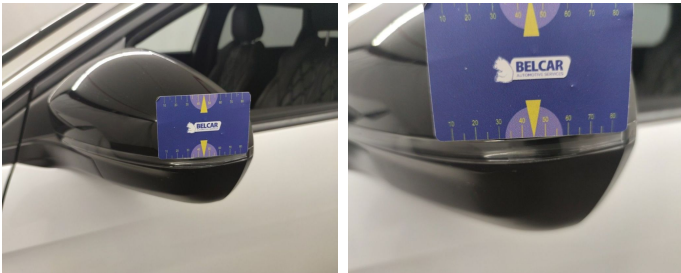
Side View Mirror Left / Direction Indicator / Replace-scratch
