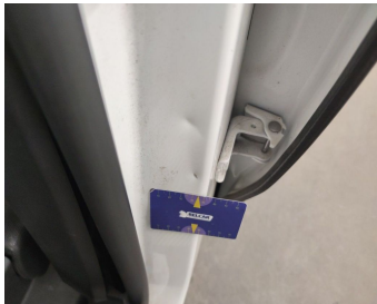
Rocker Panel Left // Smart Repair Medium-scratch + dent
