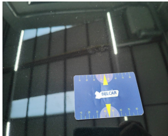
Door Rear Right // Repair & Painting-scratch + dent
