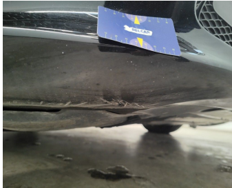
Bumper Front // Smart Repair Large-scratch
