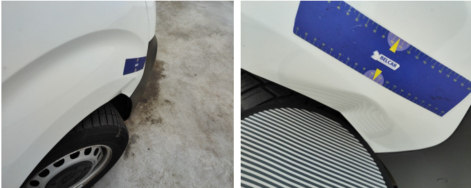
Wing Front right // Repair & Painting-dent
