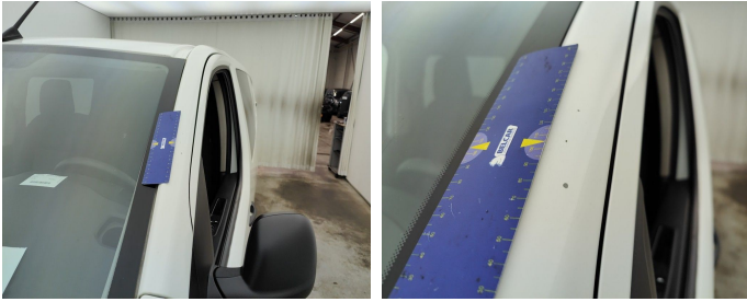
Roof // Smart Repair Medium-stone chipping
