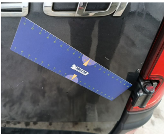
Rear Loading Door Right // Painting-scratch
