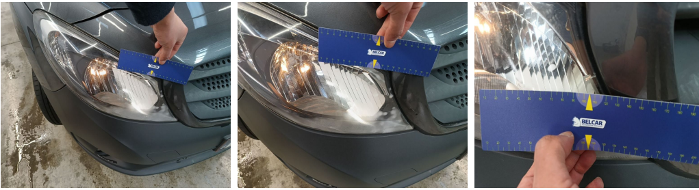
Light / Front Right / Replace-cracked
