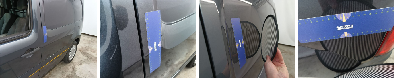
Wing Rear Left // Smart Repair Large-scratch + dent
