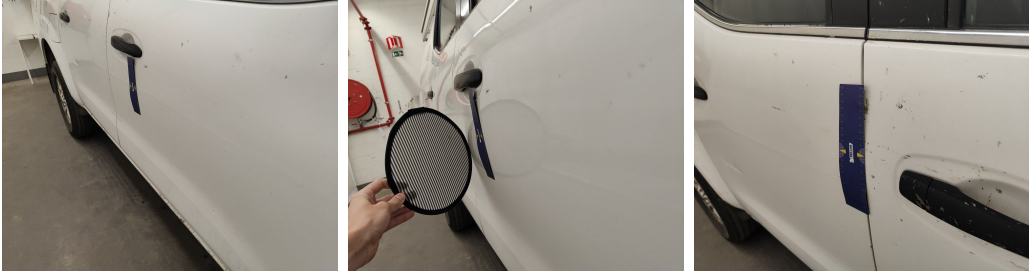
Door Front Right // Repair & Painting-dent
