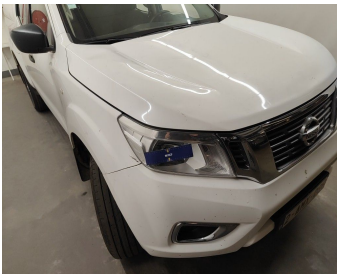
Light / Front Right / Replace-scratch
