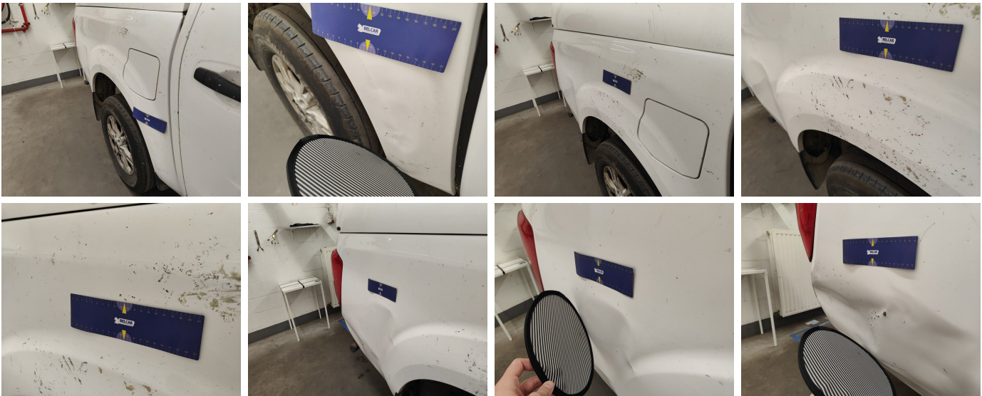
Wing Rear Right // Repair & Painting-scratch + dent
