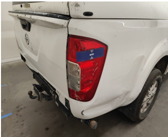
Light / Rear Right / Replace-cracked
