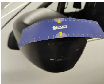
Side View Mirror Left / Shell / Replace Not Painted-stain
