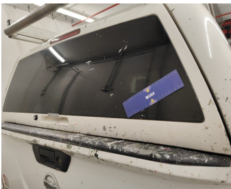
Rear Bonnet / Rear Window / Replace-scratch
