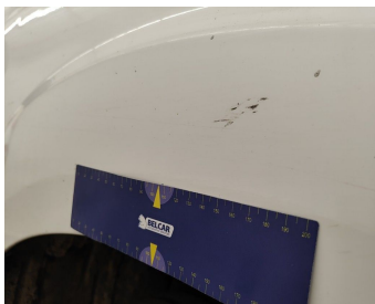
Side View Mirror Left / Shell / Replace Not Painted-stain
