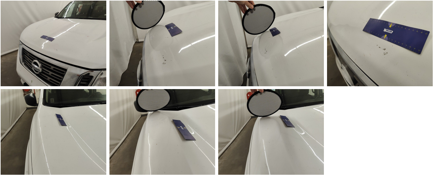
Front Bonnet // Repair & Painting-dent
