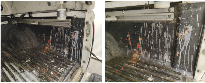
Trunk Compartment / Side Cover Right / Replace-stain
