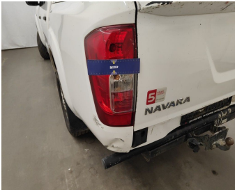
Light / Rear left / Replace-scratch
