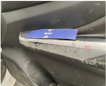
Front Right Door Interior Coating // Repair-stain
