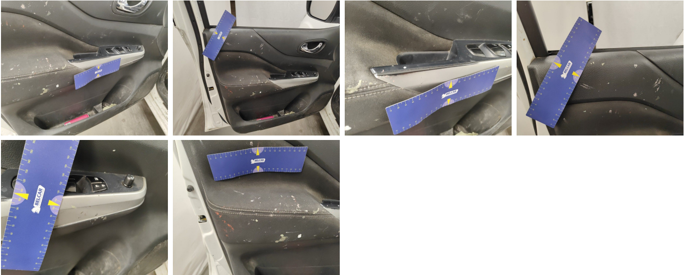
Front Left Door Interior Coating // Replace Completely-scratch
