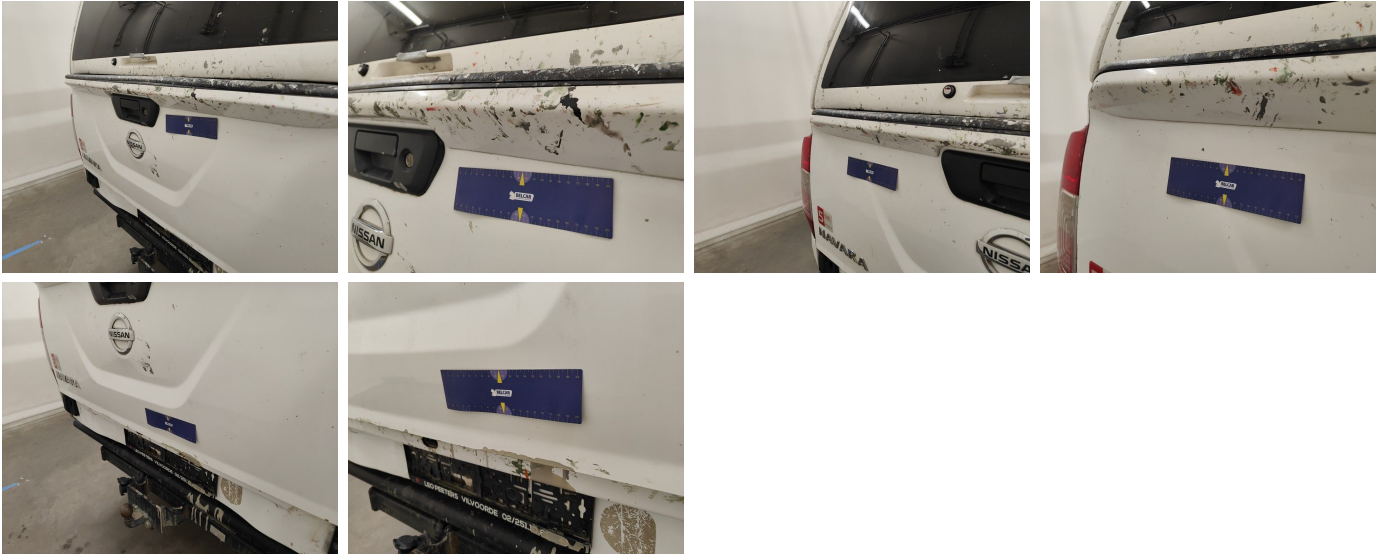
Rear Loading Door Left // Painting-Chipped paint
