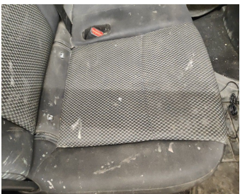
Seat Rear Right / Bottom Coating / Replace-stain
