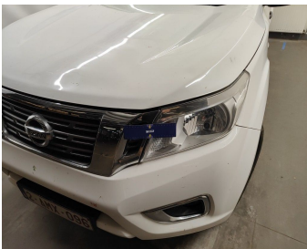
Light / Front Right / Replace-scratch
