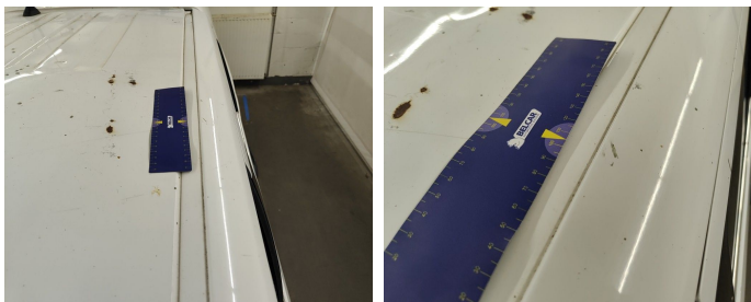
Roof // Smart Repair Medium-scratch
