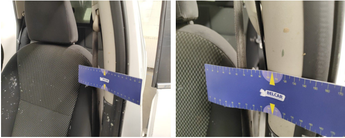
Interior / A Pillar Upper Cover / Replace-stain
