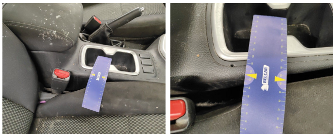
Central Console / Cup Holder / Replace-hole
