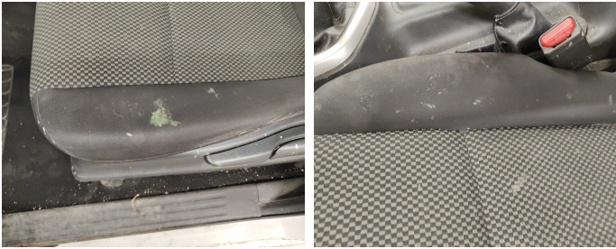
Seat Front Left / Bottom Coating / Replace-stain
