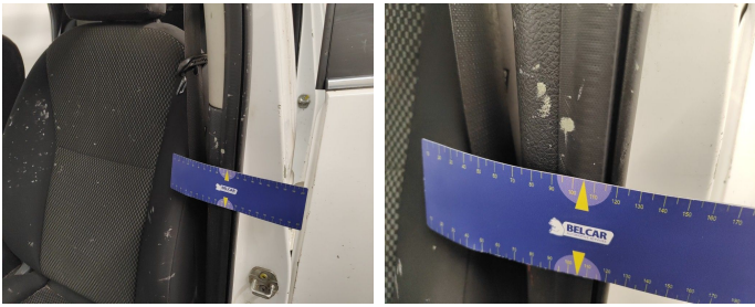
Door Front Left / Trim / Replace-stain
