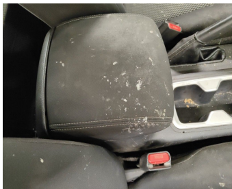
Central Console / Cover Armrest / Replace Cover Armrest-stain
