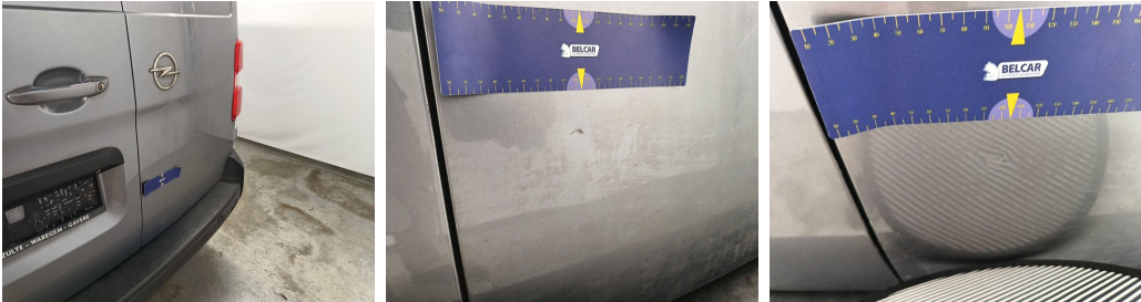
Rear Loading Door Right // Repair & Painting-scratch + dent
