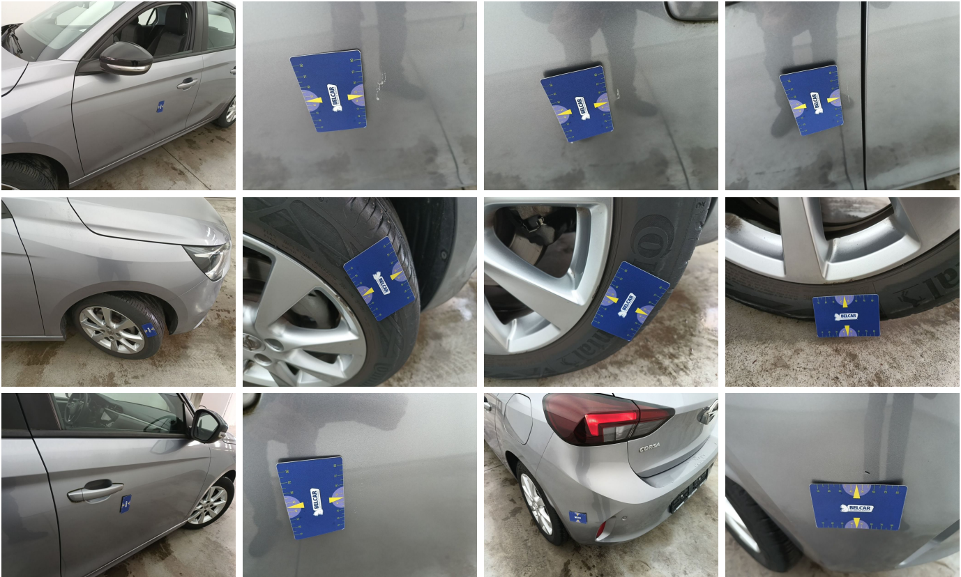
Damage within Renta-norm-scratch
