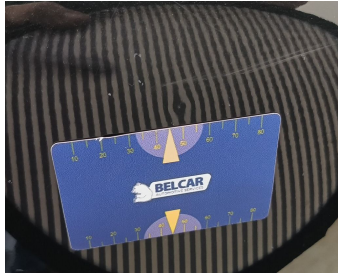
Wing Rear Right // Repair & Painting-scratch + dent
