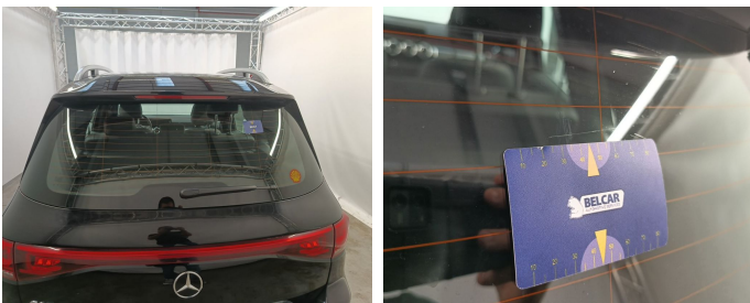
Rear Bonnet / Rear Window / Replace-scratch
