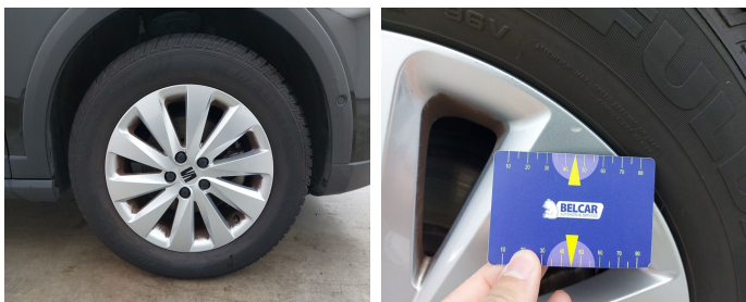
Wheel Alloy Front Right // Repair-scratch
