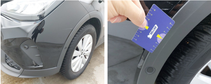
Wing Front Left / Trim / Replace-scratch
