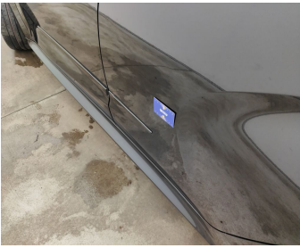
Door Rear Left // Painting-scratch + dent
