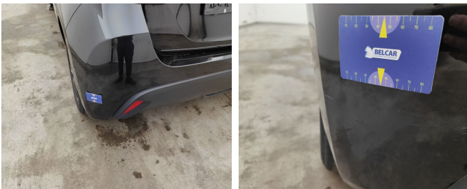
Bumper Rear // Painting-scratch
