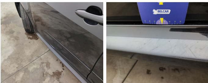
Rocker Panel Left / Cover Not Painted / Replace-scratch
