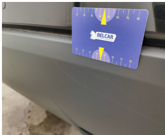
Bumper Rear / Trim Center / Replace-scratch
