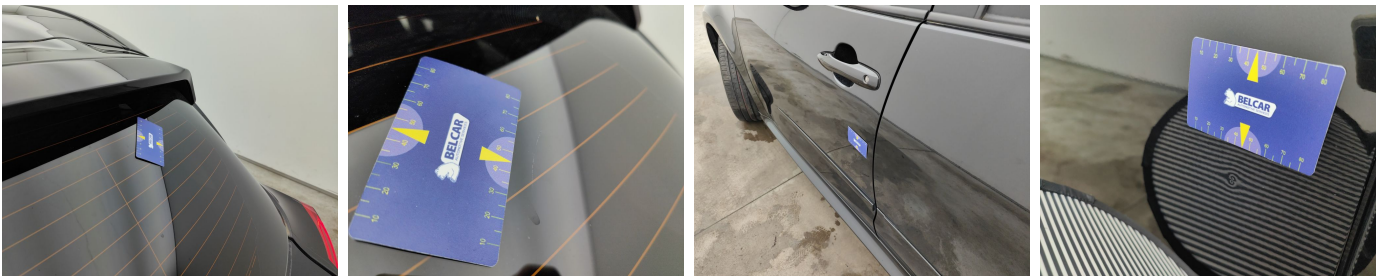
Damage within Renta-norm-scratch
