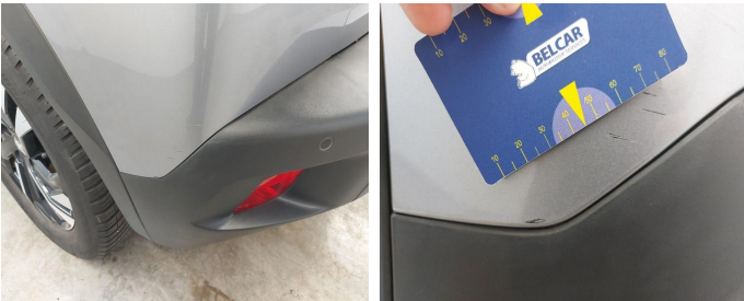
Bumper Rear // Smart Repair Medium-scratch
