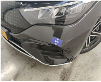
Bumper Front / Grid Left / Replace-cracked
