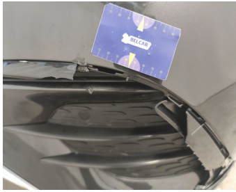
Bumper Front / Grid Left / Replace-cracked
